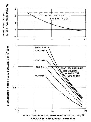
Figure 4. Effect of shrinkage and pressure differential on desalinization characteristics
