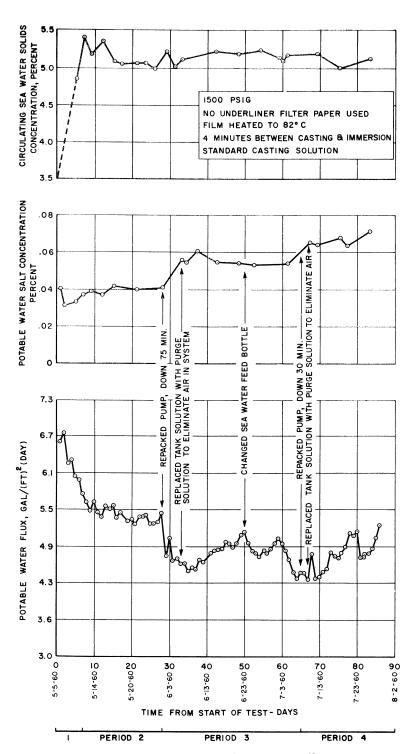
Figure 8. Life test of laboratory-cast film
