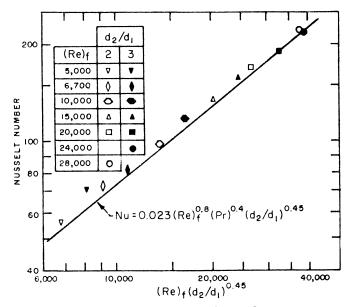
Figure 2. Heat transfer without vibration
