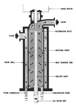
Figure 1. Schematic diagram of distilling unit
