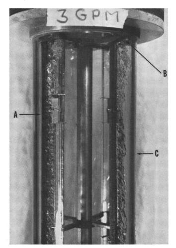
Figure 3. High speed strobe light photograph of wiper assembly in operation
