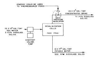
Figure 11. Proposed flow diagram of 10,000,000gallon-per-day plant
