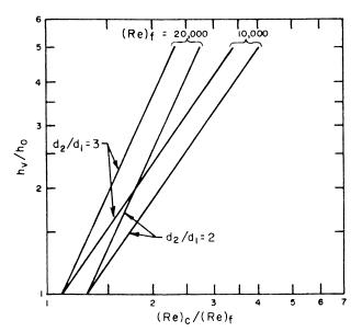
Figure 3. Heat transfer with vibration
