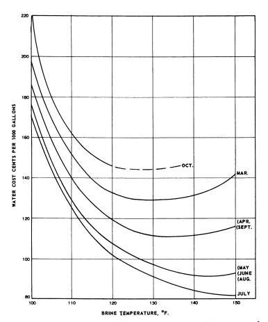
Water cost vs. brine temperature for 3° F. terminal Figure 10. temperature difference
