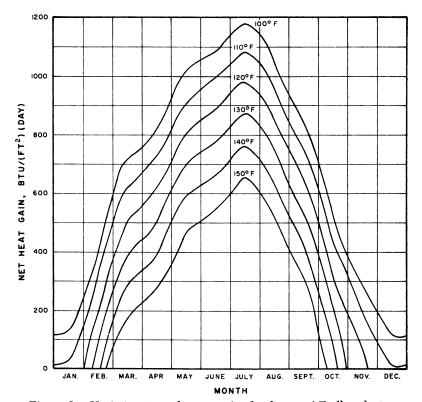
Figure 6. Variation in net heat gain for five layers of Tedlar glazing
