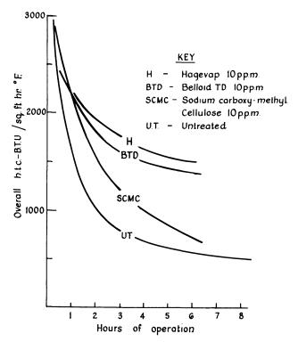
Figure 4. Over-all heat transfer coefficient vs. time for sea water plus commercial additives
