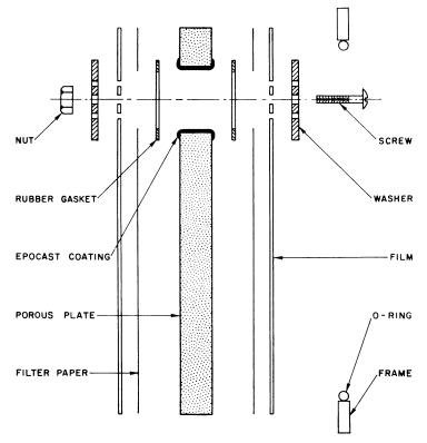
Figure 10. Dissassembled package-frame assembly of 4-inch desalinization cell
