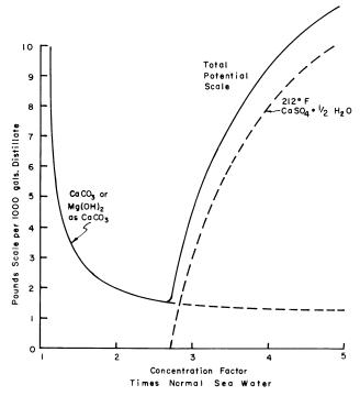
Figure 2. Potential scale from normal sea water
