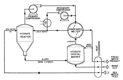
Figure 5. Flowsheet of hydrate process for desalting sea water
