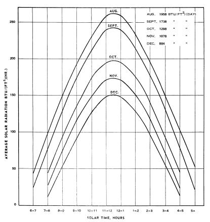
Figure 3. Average hourly solar radiation on a horizontal surface
