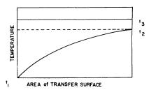
Figure 2. Temperature difference in evaporators
