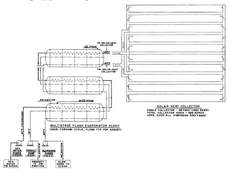
Figure 1. Schematic flow diagram 3° F. terminal temperature difference
