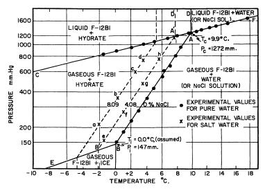
Figure 3. Experimental phase diagram for F-12B1-water-NaCl system
