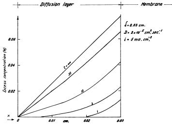
Figure 5. Concentration profile in boundary layer
