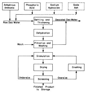
Figure 1. Process flowsheet for descaling sea water and producing fertilizer
