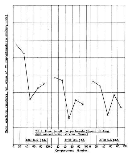
Figure 6. Distribution of electrical resistance across 100-compartment pack, and effect of over-all flow rate
