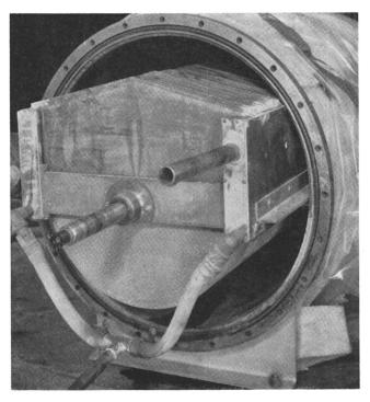
Figure 8. Flat plate condenser and rotating disk assembly in multistage test unit
