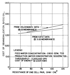
Figure 4. Effect of resistance of a cell pair on cost of demineralization
