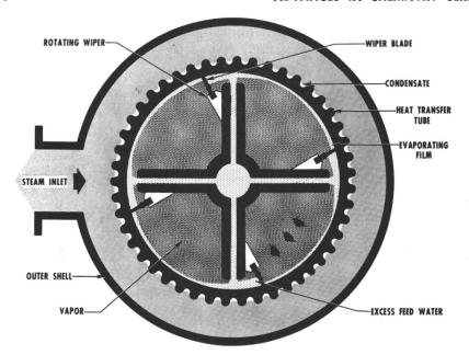
Figure 2. Operation of thin-film distilling unit
