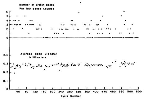
Figure 8. Dowex 50W particle size during pilot plant operation
