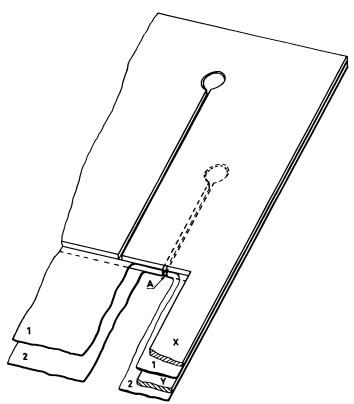
Figure 5. Mechanism of slot or intercompartmental leakage
