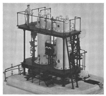
Figure 8. Distillation pilot plant Office of Saline Water, 37,000 gallons per day
