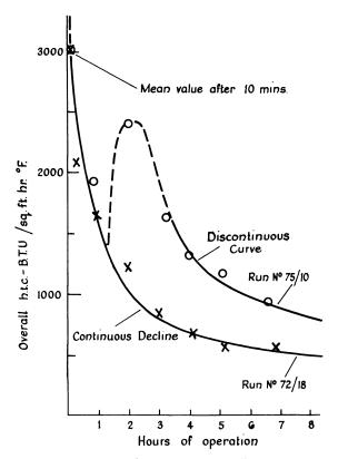
Figure 2. Over-all heat transfer coefficient vs. time for untreated sea water
