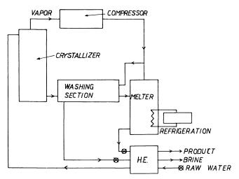
Figure 6. Block diagram of freezing evaporation pilot plant
