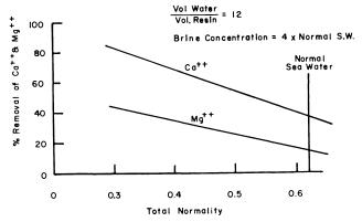
Figure 11. Removal of calcium and magnesium from sea waters
