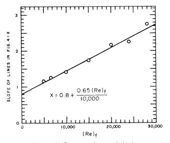
Figure 5. Change of slope with  $(Re)_t$
