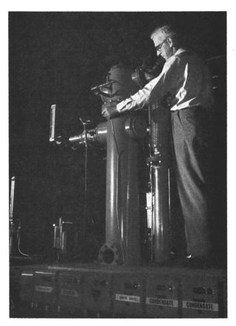
Figure 6. Wiped thin-film distilling unit
