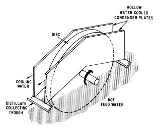
Figure 2. Schematic diagram of diffusion still
