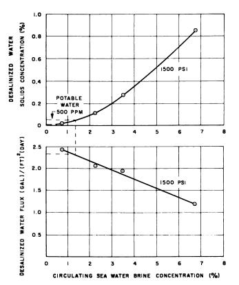
Figure 5. Effect of sea water solids concentration on desalinization characteristics
