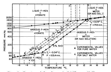
Figure 1. Experimental phase diagram for F-142b-water-NaCl system
