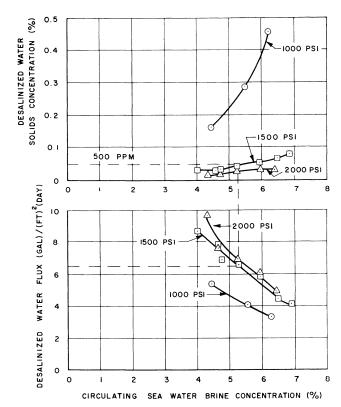
Figure 7. Effect of sea water concentration on desalinization characteristics
