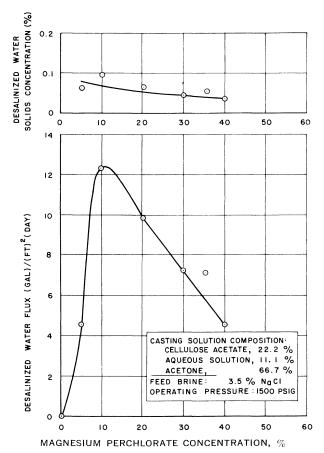
Figure 6. Effect on film performance of percentage of magnesium perchlorate in aqueous solution
