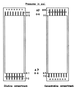
Figure 7. Pressure drop across and pressure differential between diluting and concentrating compartments for 30 U. S. gallons per hour per compartment
