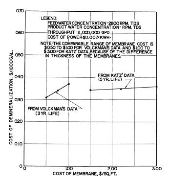
Figure 2. Effect of cost of membranes on cost of demineralization
