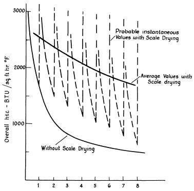
Figure 3. Over-all heat transfer coefficient for untreated sea water with scale drying
