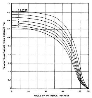
Figure 4. Transmittance-absorption product for Tedlar glazing and black-bottom surface with respect to angle of incidence
