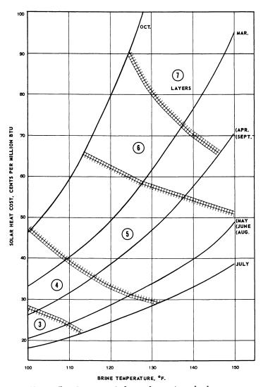
Figure 7. Domains of glazing layers for solar heat cost
