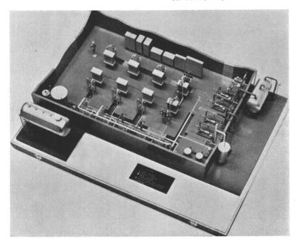
Figure 1. Model of 650,000-gallon-per-day Ionics electrodialysis desalting plant
