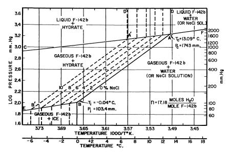
Figure 2. Calculated phase diagram for F-142b-water-NaCl system
