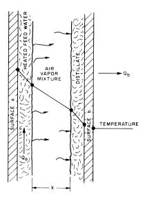
Figure 1. Basic principle of diffusion
