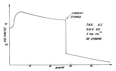
Figure 3. Electric potential drop across membrane vs. time Anion exchange membrane (T.N.O., The Hague, Netherlands) Solution 0.01 N KCl. Current density 5 ma. per sq. cm. No stirring. Experiment carried out in apparatus shown in Figure 2
