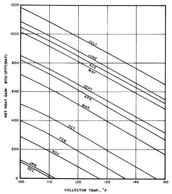
Figure 5. Net heat gain for five layers of Tedlar glazing
