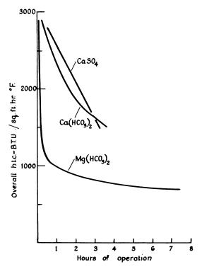
Figure 5. Over-all heat transfer coefficient vs. time for synthetic scaling solutions
