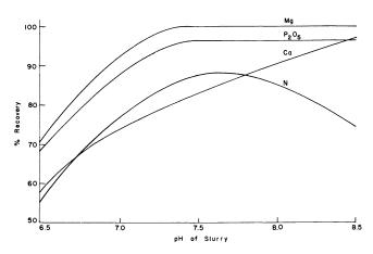
Figure 5. Effect of pH on recovery
