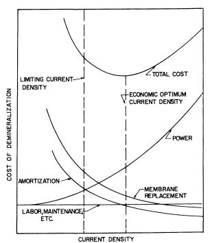
Figure 1. Factors making up total cost of demineralization by electrodialysis for a typical installation
