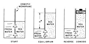
Figure 1. Principle of osmotic desalinization
