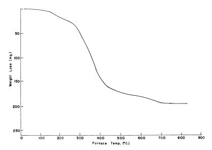
Figure 3. Thermogram of fertilizer from sea water
