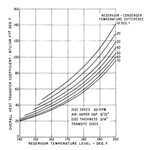
Figure 5. Condenser component performance
