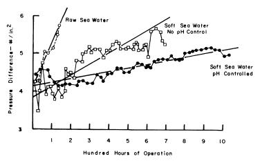
Figure 12. Increase in evaporator pressure difference with time of operation
