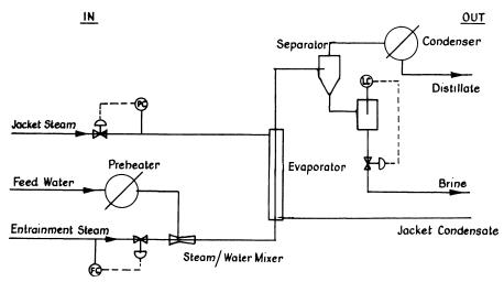
Figure 1. Simplified flow diagram for spray evaporation plant
