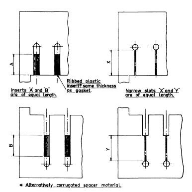
Figure 8. Alternative gasket slot feeding arrangement for equalizing pressure drop and supporting membrane
