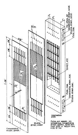
Figure 4. Electrode and intermediate plates, gaskets, and spacer design
