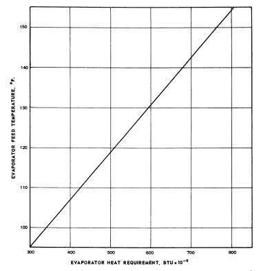
Figure 9. Variation in heat requirements of flash evaporator with brine feed temperature
