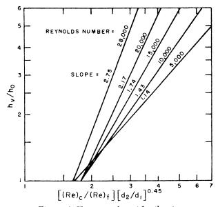
Figure 4. Heat transfer with vibration
