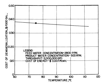
Figure 5. Effect of temperature on cost of demineralization
