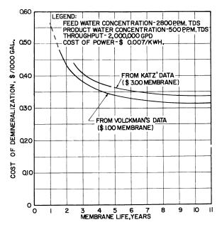
Figure 3. Effect of membrane life on cost of demineralization
