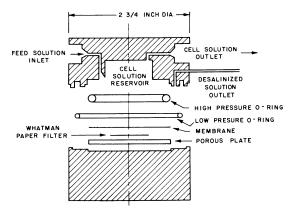
Figure 2. Diassembled view of small desalinization cell
