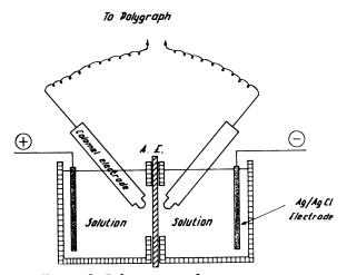
Figure 2. Polarization voltage measurement
