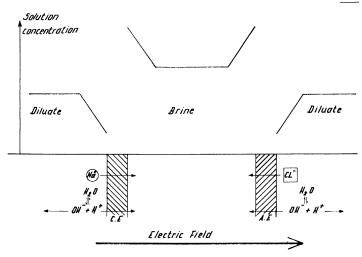
Figure 1. Steady-state concentration profiles near membrane surfaces in electrodialysis
