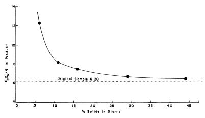
Figure 2. Effect of slurry concentration on decomposition during dehydration
