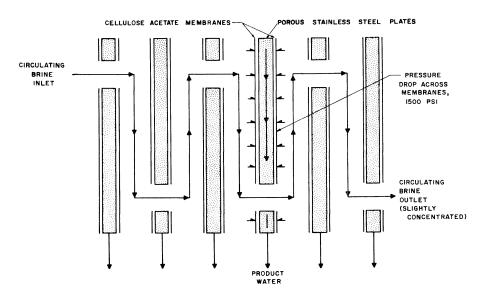
Figure 9. Flow through film packages
