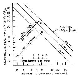
Figure 1. Stability diagrams and evaporation paths of CaSO<sub>4</sub> in sea water
