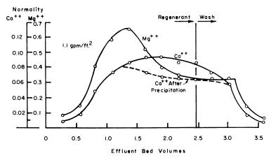
Figure 7. Typical regeneration wave
