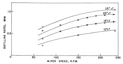
Figure 4. Marine tube performance Evaporating temperature level 170° F.
