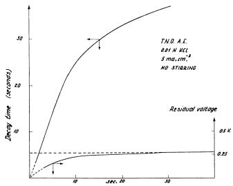
Figure 4. Decay time and residual voltage vs. current time Materials and conditions as described in Figure 3
