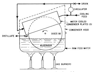
Figure 3. Single-stage bench model
