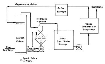
Figure 5. Flowsheet of soft sea water pilot plant
